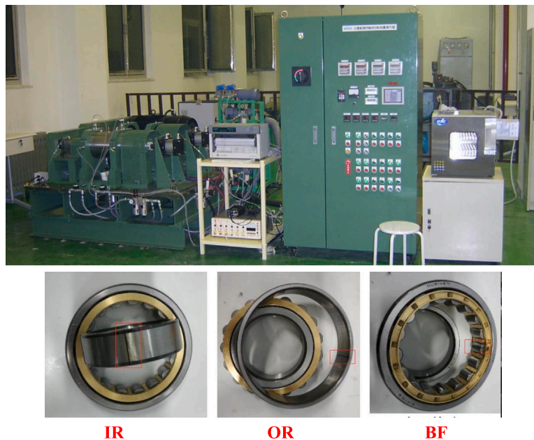
Fig. 9. High-speed train traction motor bearing platform.
